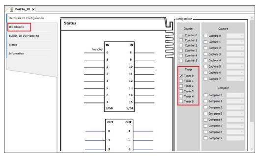
2. The following is an example of the configuration function. For the axis name used in the POU, Timer\_0 is required.
