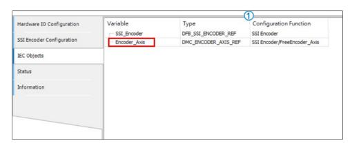
3. For the **MC\_CamIn** function block in the POU, the source of the spindle can use SSI as the source. The input axis name is Encoder\_Axis.
