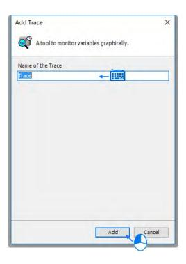
3. After the Trace is successfully added, it will be shown in the project tree on the left side of the screen. Then double click on "Trace" to open the Trace page.
