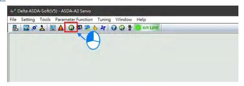
6. As shown in the following figure, the field being circled by the red box on the upper part of the page displays all the servo parameters in groups.
