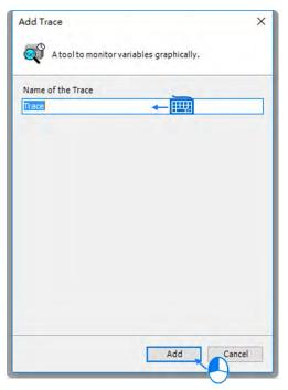
3. After the Trace is successfully added, it will be shown in the project tree on the left side of the screen. Then double click on "Trace" to open the Trace page.
