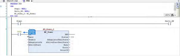
16. Insert the name of servo drive to the Axis input pin of the function block and delete "???" of other pins, since the mark "???" does not represent any variables and errors may occur while parsing.
