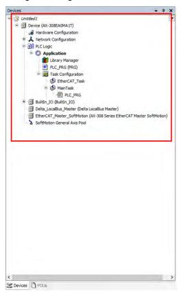
7. Double click on "Network Configuration" to create servo axes in the system.
