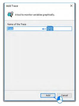
2. After the Trace is successfully added, it will be shown on the project tree on the left side of the screen. Then double click on "Trace" to open the Trace page.
